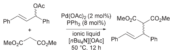
Scheme 5 Palladium catalysed allylic alkylation reaction.
